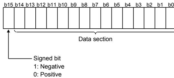
3.4.8 Write data error codes (buffer memory address 19: Un\G19)
