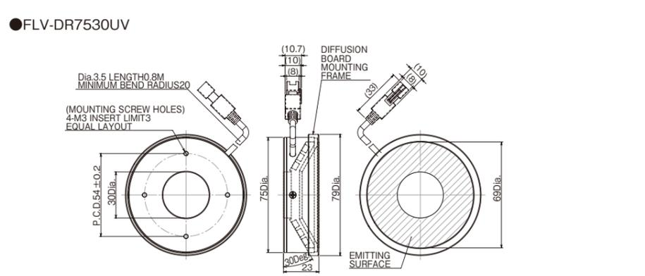
Tightening torque: 0.54N · m
