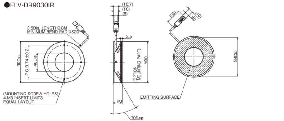
Tightening torque: 0.54N · m
