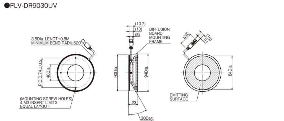
Tightening torque: 0.54N · m
