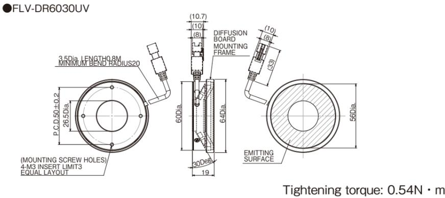
Tightening torque: 0.54N · m
