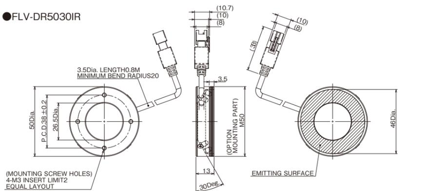
Tightening torque: 0.54N · m
