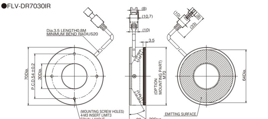
Tightening torque: 0.54N · m
