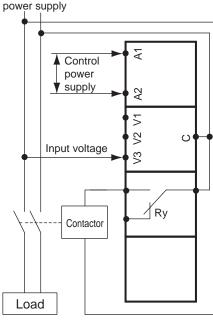
Connect the input between terminals V1-COM, V2-COM, V3-COM depending on the input voltage
