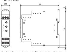
Installation Procedure: Attaching to the DIN rail or attaching with front screws Measurements for attachment with front screws
