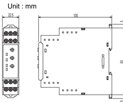
\*Installation Procedure : Attaching to the DIN rail or attaching with front screws
