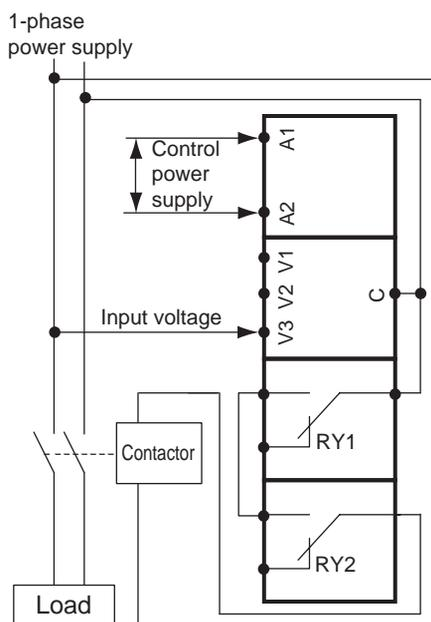
\* Connect the input between terminals V1-COM, V2-COM, V3-COM depending on the input voltage
