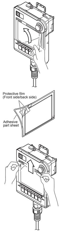
1) Remove the old protective sheet from the GOT holding the lower right corner, and clean the GOT surface.
