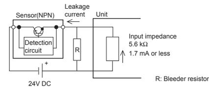
$$R(k\Omega) < 1.7(mA) / \text{Leakage current}(mA) - 1.7(mA) \times 5.6(k\Omega)$$
