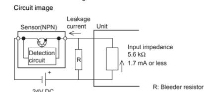
$R(k\Omega) < 1.7(mA) / \text{Leakage current}(mA) - 1.7(mA) \times 5.6(k\Omega)$
