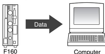
1. Connect the RS-232C cable to the COM1 port on the personal computer and the RS-232C/422 connector on the F160.
