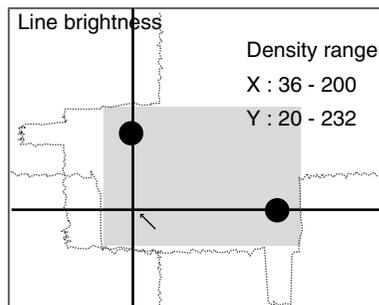
5. Move the solid line to the desired position for observing density distribution. Use the **Up/Down** Keys to move the horizontal line. Use the **Right/Left** Keys to move the vertical line.
