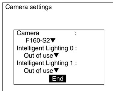
2. Select the model of the connected Camera.
