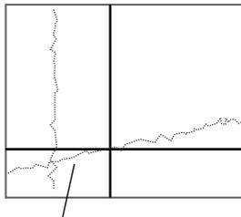
If a homogeneous color is being displayed but the graph has an incline, it indicates that the lighting is uneven.
