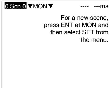
**CHECK** When the settings have been completed, it is useful to use Startup Mode when actually operating the F160. Startup Mode is used to set the startup conditions (display screen) when the F160 is next started. For example, set the F160 to start in Run Mode. This will allow measurements to be started immediately and will make day-to-day operations easier. (Refer to page 118.)
